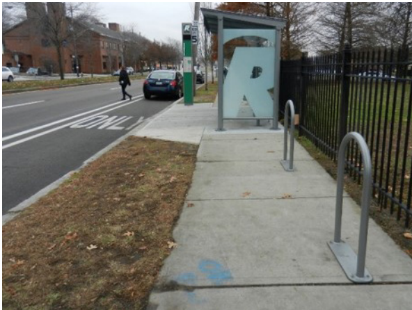
Inverted U style bike rack at RIPTA stop on North Main Street, Providence, RI
