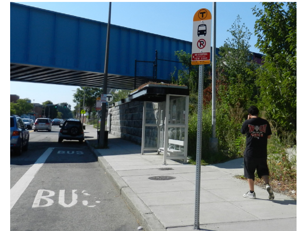
Narrow style shelter with standard roof size and a green roof in Boston, MA
