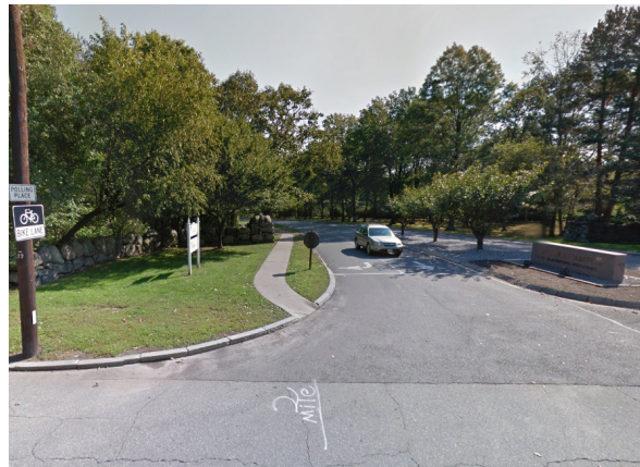
RIPTA stop on Blackstone Boulevard at the entrance to Butler Hospital Campus in Providence, RI has no landing area or sidewalk connection. On the other side of the driveway lies the path to the campus; no crosswalk connects the stop and the path
