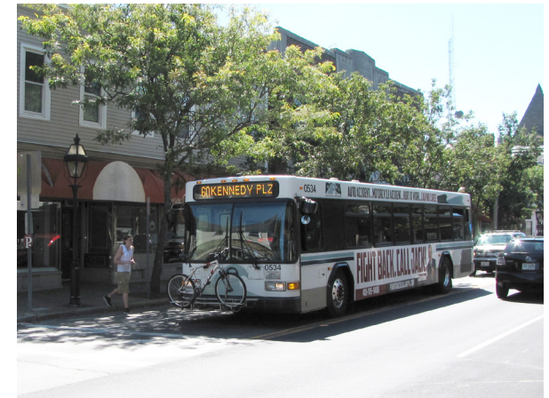
A vehicle parks in the RIPTA stop on Route 114 at Child Street/Route 103 in Warren, RI forcing bus operators to stop in the travel lane, far from the curb, and riders to step into the roadway to access the bus. Bus stop striping, and a no parking sign at the rear of the stop, would help to better define the bus stop limits
