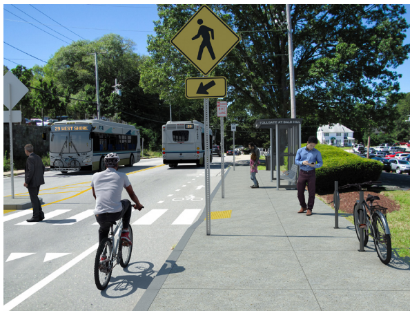
Figure 5.4 Striping at a Conceptual RIPTA Bus Stop in Bike Lane on Toll Gate Road at Bald Hill Road in Warwick, RI
