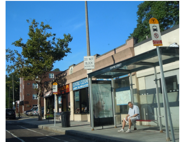
Curb extension at an MBTA bus stop in Boston, MA allowed for the retention of an existing tree and the addition of rider amenities. Abutters added to the aesthetics with planters
