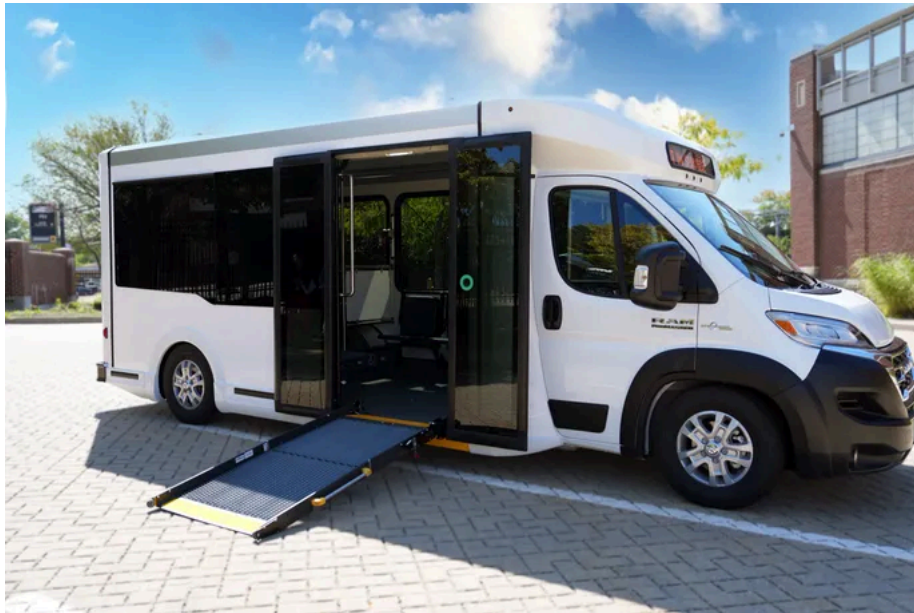
The new Model 1 Ride Paratransit van with doors open and wheelchair ramp extended.
